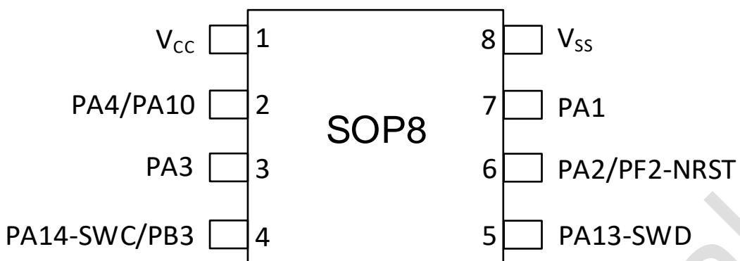
图 3-7 SOP8 Pinout1 PY32F002AL15Sx
