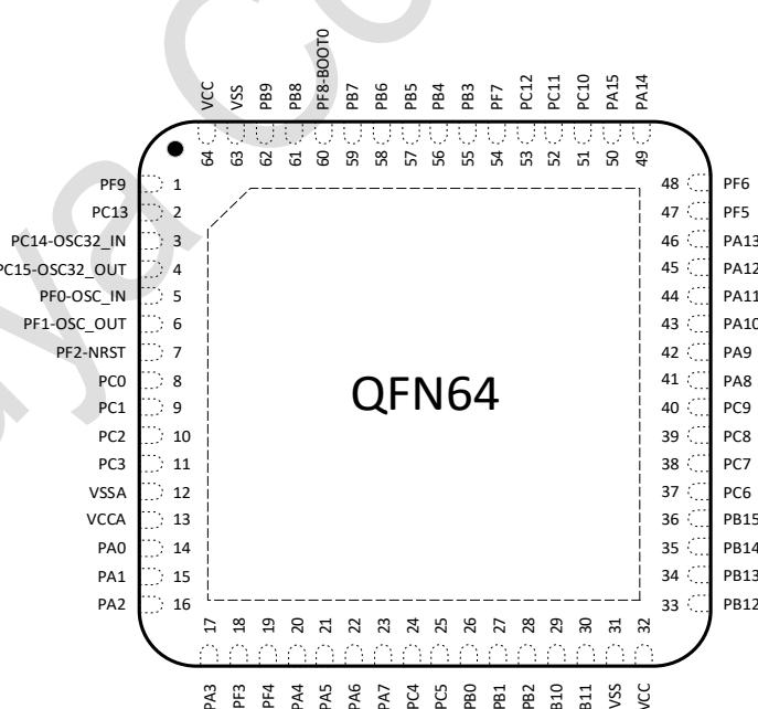
图 3-2 QFN64 PY32F071R1xU6 Pinout1 (Top view)
